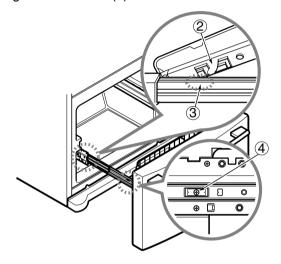
With the drawer pulled out to full extension, insert the lower basket (5) in the rail assembly until it doesn't move forward.
